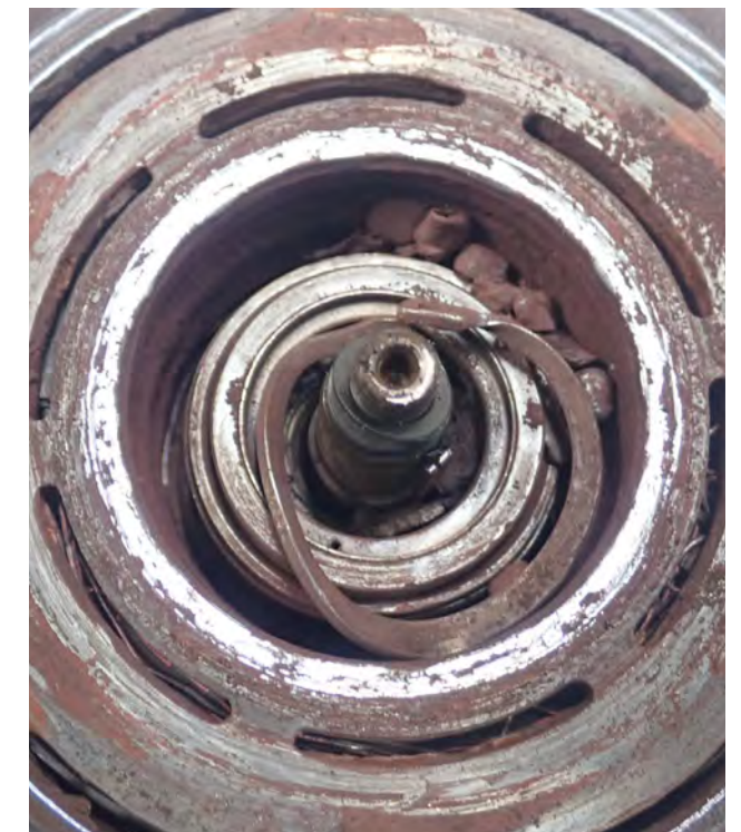
Abb. 2 Kugellager defekt
