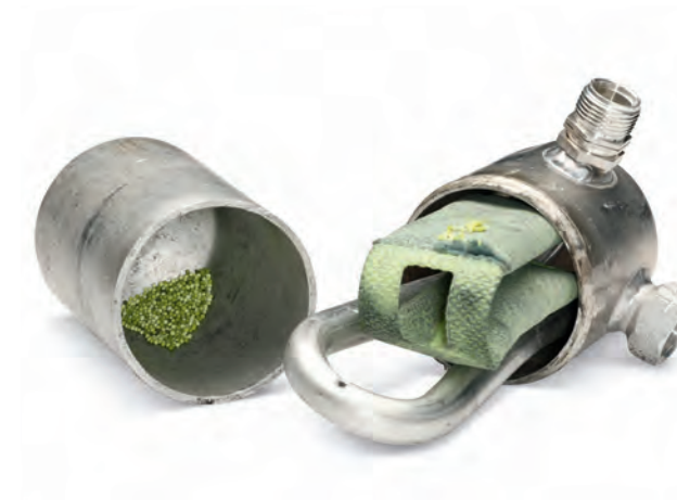
Abb. 1 Granulataustritt Filter-Trockner
